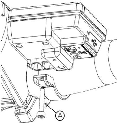
3. Open the clamps of controller panel and place it on to the handlebar in the correct position. Now with M4\*12 screws (A) tighten the controller panel onto position. Torque requirement: 1N.m.
