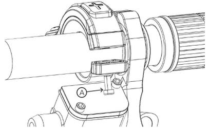
4. Link the cable from controller panel (B) and the cable from E-Bus (A) onto the display.
