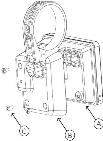
2. Open the clamps of display and place the display on to the handlebar in the correct position. Now with M3\*14 screws (A) tighten the display into position. Torque requirement: 0.3N.m.
